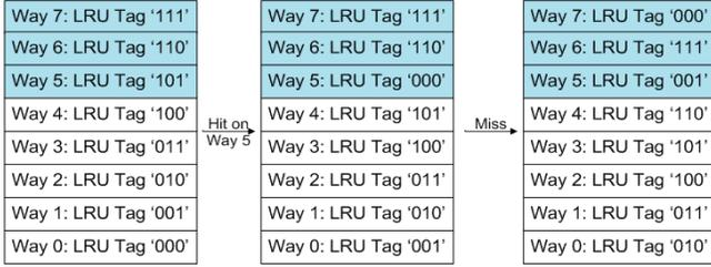
Fig. 3. Conventional LRU replacement scheme allows data to be mapped to long latency cache blocks.
