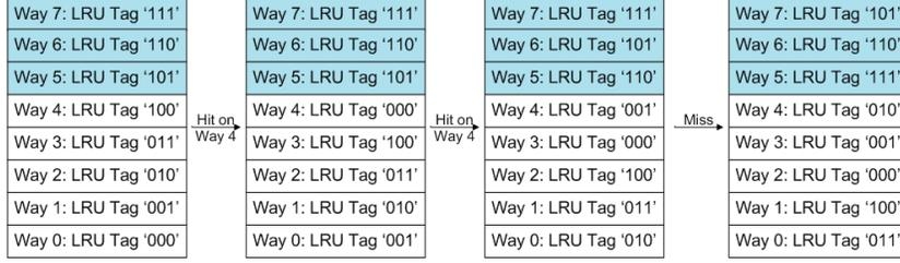
Fig. 4. On a hit, LA-LRU switches the data and the tag of the high latency block with a low latency block, so as to migrate the frequently accessed data to the low latency blocks.
