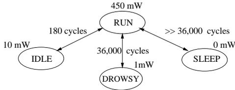
Figure 2: Power State Machine of XScale
