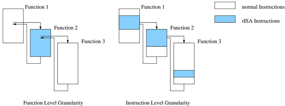
Fig. 6. Routine Level Granularity versus Instruction Level Granularity
