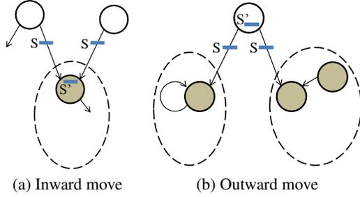
**Figure 5.** Moving mode change operations from edge to node for save operations. Solid circles represent nodes, or basic blocks (white: mode A, gray: mode B), and dashed ovals represent selected maximal AFRs. Thick small bars represent save operations ( $S$ : before move,  $S'$ : after move).
