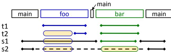
**Figure 3.** Vulnerable intervals of the example, represented by solid bars. The dashed bar in the last row is not vulnerable. Among the four round boxes indicating the intervals that would be protected by ad-hoc method, only one ( $s1$ ) is vulnerable.
