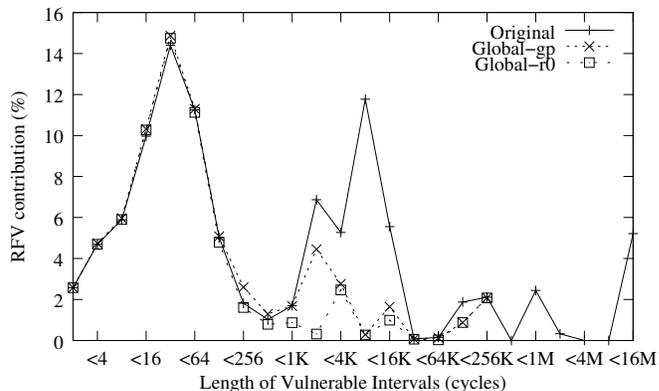
**Figure 7.** Comparing RFV distributions before/after the proposed optimization.
