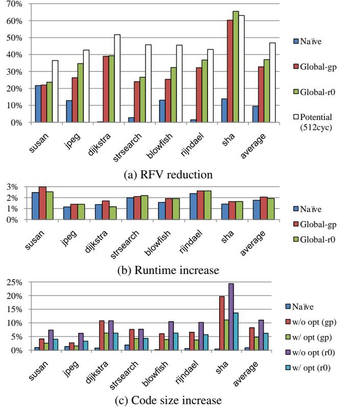
**Figure 6.** Comparing different approaches in terms of RFV, runtime, and code size.
